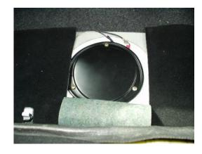
At this point you will be looking directly at the top of the diesel tank and the fuel sender
